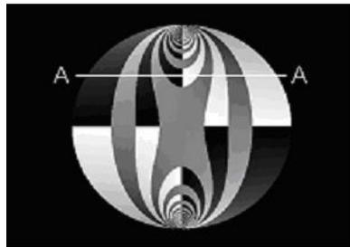
**Figure 7. Phase Maps of Isoclinic from Simulation of a Disk under Diametric Compression**
