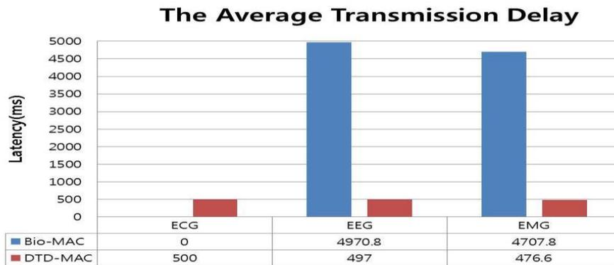
**Fig. 4.** Comparison of the average transmission delay on the transmission of various biological signal
