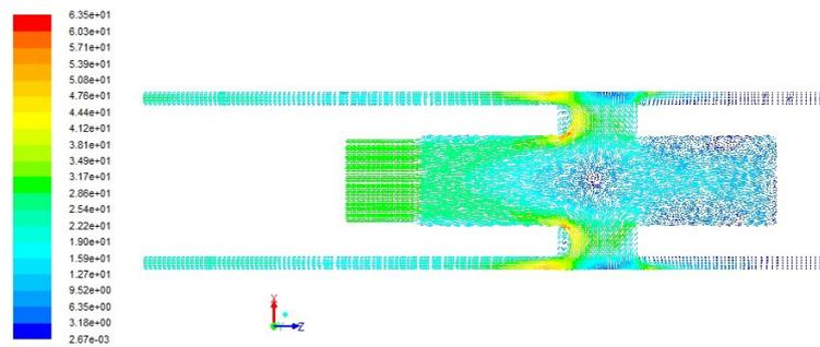
**Fig. 2.** Velocity vector of plane (Y=0).
