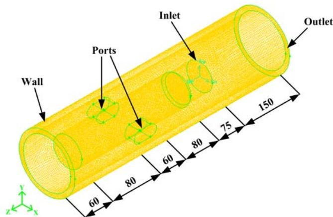
Fig.1. Mesh generation of the fracturing sleeve geometry.
