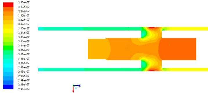
**Fig. 3.** Pressure contour of plane (Y=0).
