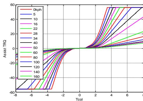
**Fig. 2.** Base assist torque map
