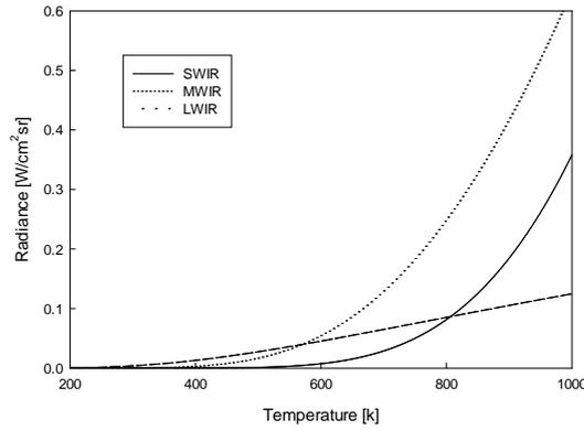
**Fig. 3.** Temperature-radiance curve for individual WBs.
