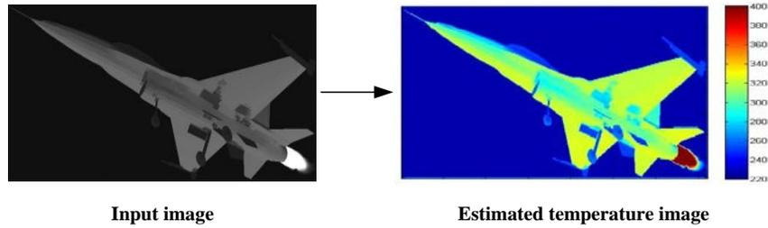
**Fig. 3.** Input image and estimated temperature image.
