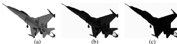
**Fig. 4.** IR target (F16) images. (a) Original LWIR; Transformed target image to (b) MWIR and (c) SWIR band.
