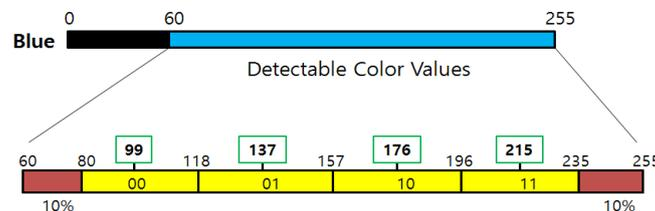
**Fig. 2.** The Digital Data Encoding Algorithm
