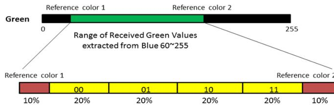
Fig.4. The color code decoding algorithm
