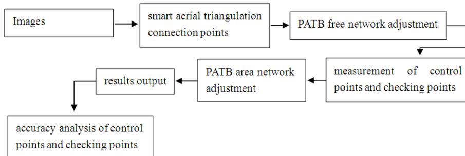
**Fig. 2.** Flow diagram of the aerial triangulation technology
