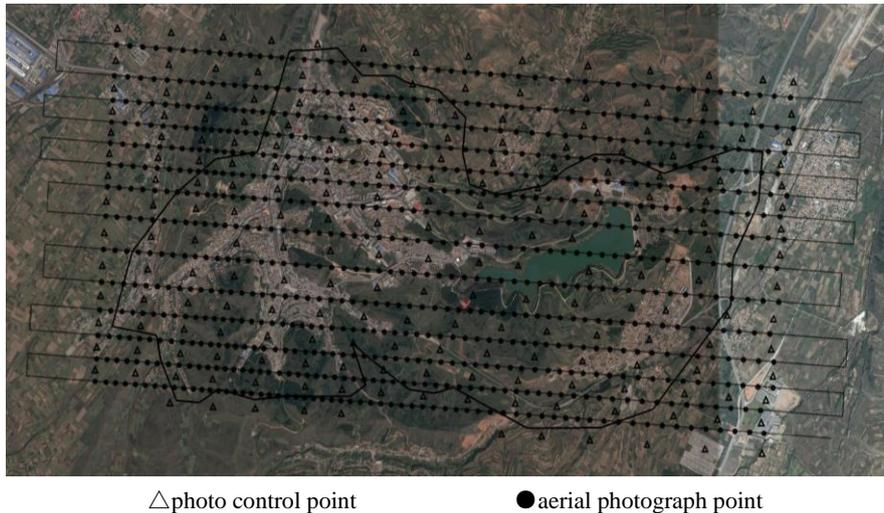
**Fig. 1.** Schematic diagram of the designed air lines
