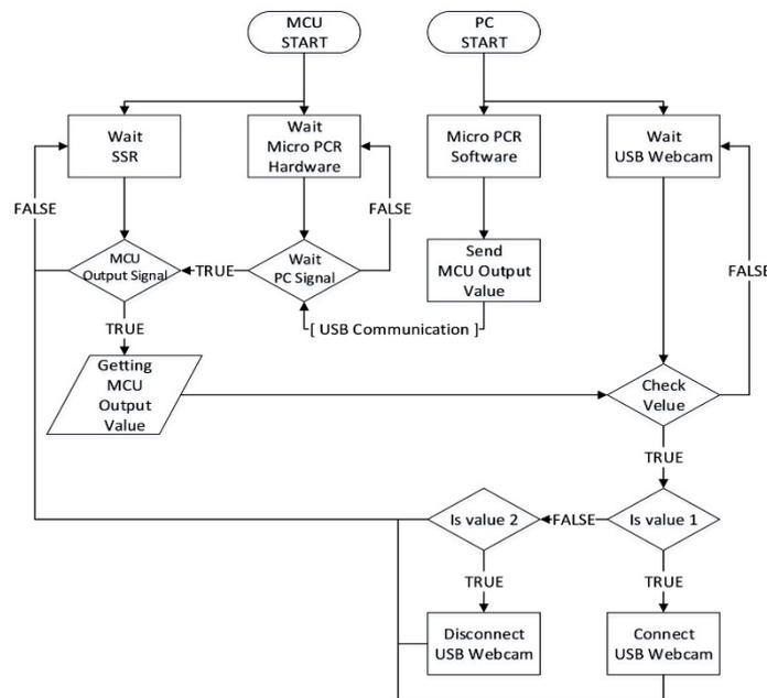
**Fig. 2.** USB Camera Operation Flow Diagram Using MCU and SSR Control
