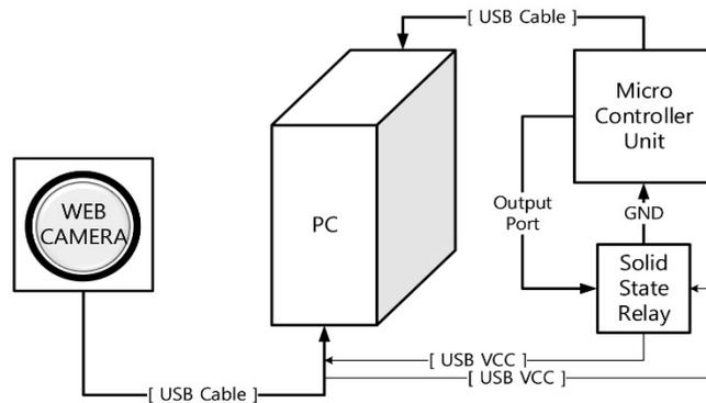
**Fig. 1.** Diagram on SSR and MCU Link of USB Webcam
