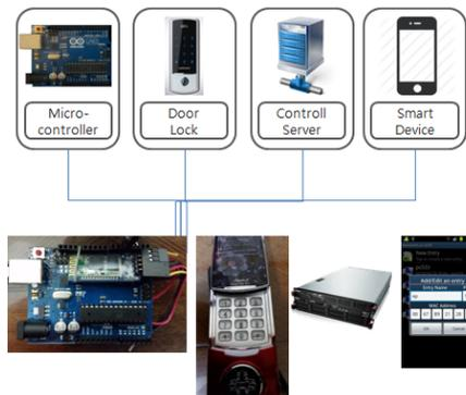
Fig. 3. Prototype of implemented access authentication system
