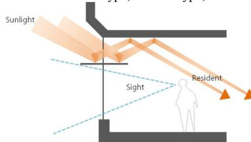
Fig. 1. The principle of the shelf system of light [1]
