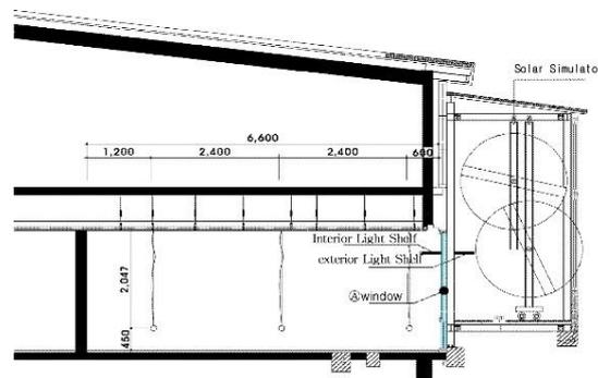
**Fig. 3.** Position of the illuminance sensor Ceiling
