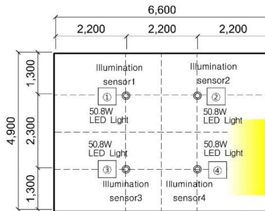
**Fig. 2.** Height of the illuminance sensor and the cross section of the test bed
