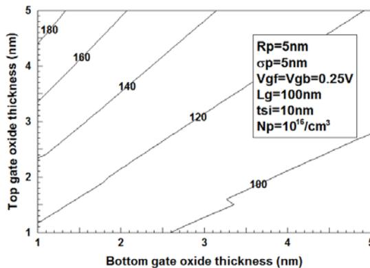
**Fig. 3.** The contours of subthreshold swings for top and bottom gate oxide thickness under the conditions of  $L_g = 100\text{ nm}$ ,  $t_{si} = 10\text{ nm}$ ,  $V_{gf} = V_{gb} = 0.25\text{ V}$  and  $N_p = 10^{16} / \text{cm}^3$ .
