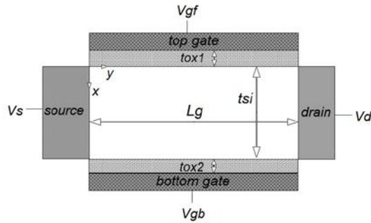
**Fig. 1.** The schematic diagram of a asymmetric DGMOSFET.
