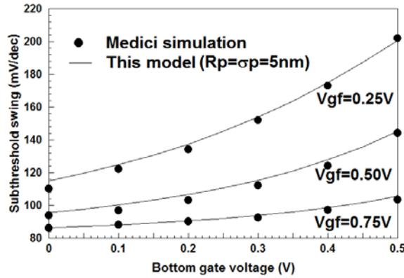
**Fig. 2.** The subthreshold swings for bottom gate voltage with a parameters of top gate voltage under the conditions of  $L_g = 25\text{ nm}$ ,  $t_{si} = 10\text{ nm}$ ,  $t_{ox1} = 1\text{ nm}$ ,  $t_{ox2} = 1\text{ nm}$  and  $N_p = 10^{16} / \text{cm}^3$ . The line describes the subthreshold swings of this model and dots are those for Medici simulation.
