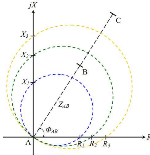
**Figure 6. Characteristic Curves of MHO Distance Relay**
