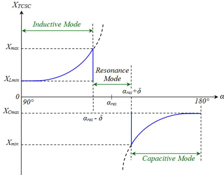
**Figure 2. Characteristic Curve  $X_{TCSC} = f(\alpha)$**
