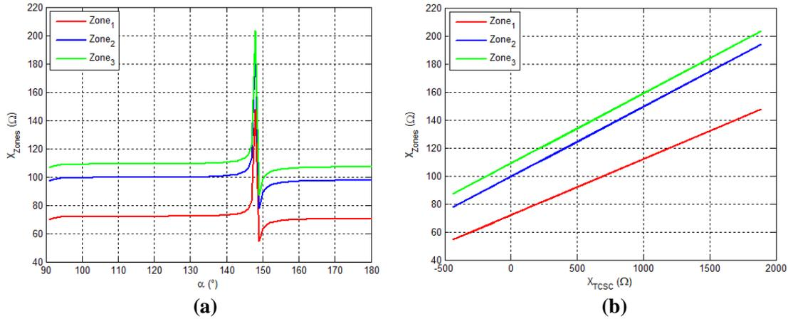
**Figure 12. Settings Zones Reactance with Respect to  $\alpha$  and  $X_{TCSC}$**
