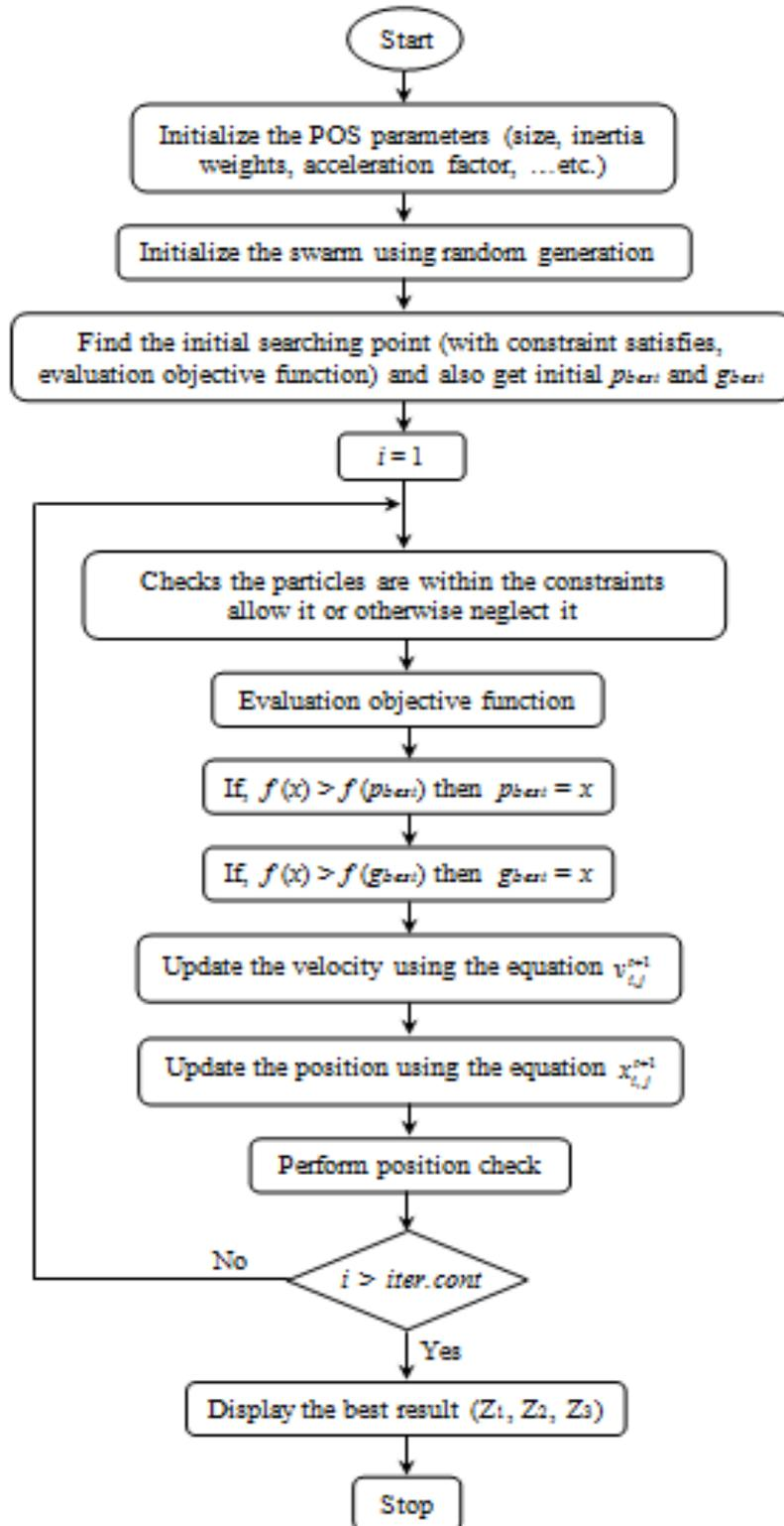
Figure 8. Flow Chart of MPSO Technique Proposed
