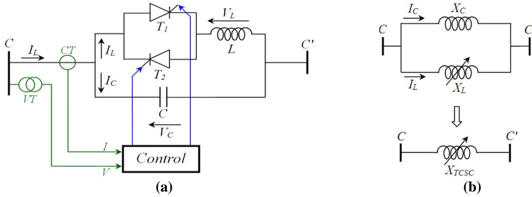
**Figure 1. Transmission Line with TCSC System:
