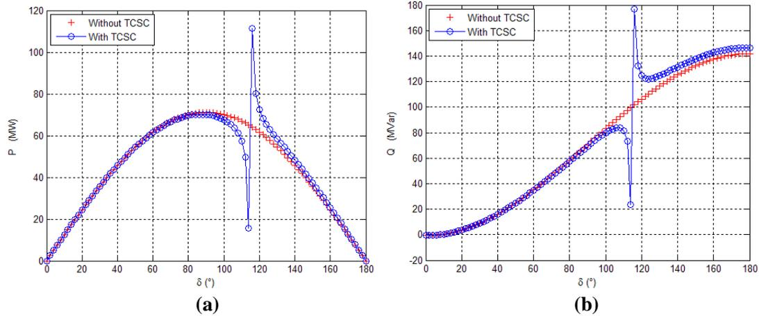
**Figure 11. Impact of TCSC on Power Transmission Line:
