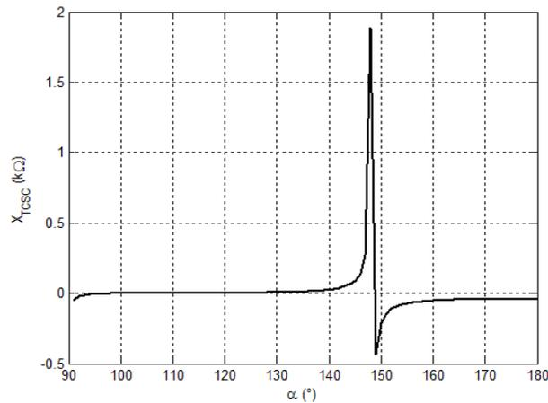
**Figure 10. Characteristic Curve  $X_{TCSC}(\alpha)$**
