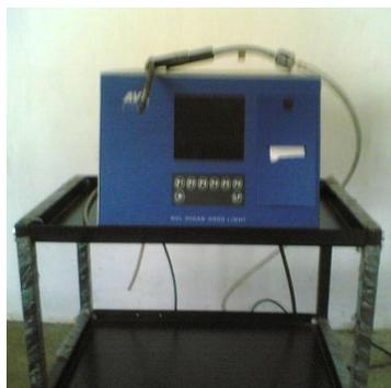
**Figure 2. AVL Five Gas Analyzer**
