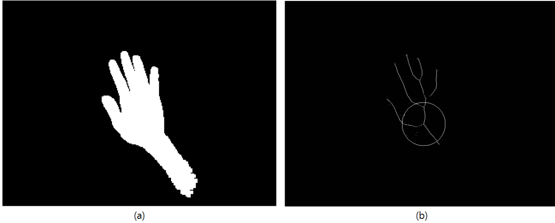
Figure 6. Hand Skeleton Extraction Example. (a) Hand Image, (b) Extracted Hand Skeleton
