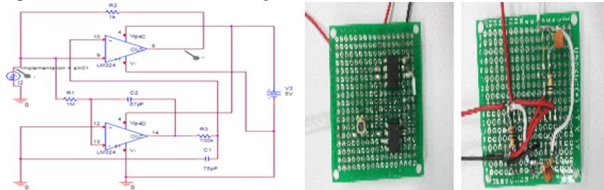
**Fig. 1.** The implement of Amplification circuit using the OP-amp
