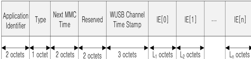
**Figure 3. The general structure of an MMC Control packet**
