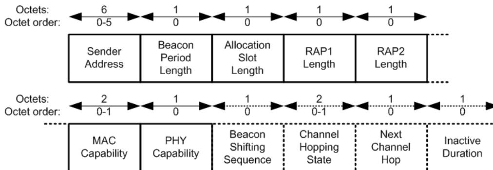
**Figure 6. WBAN beacon frame format**
