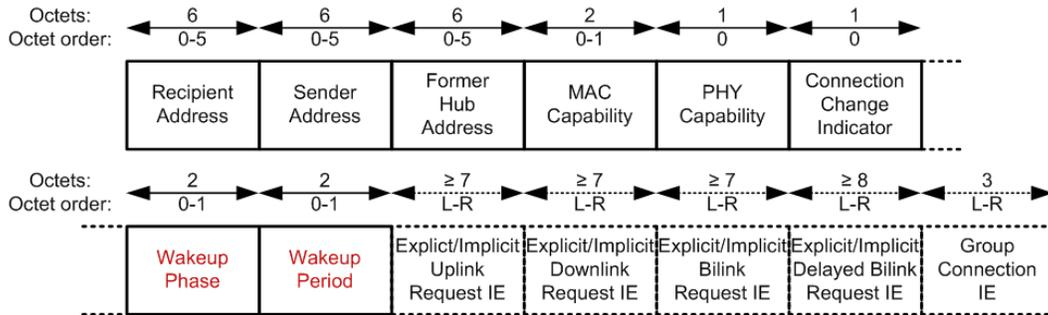
**Figure 8. Connection Request control frame format**
