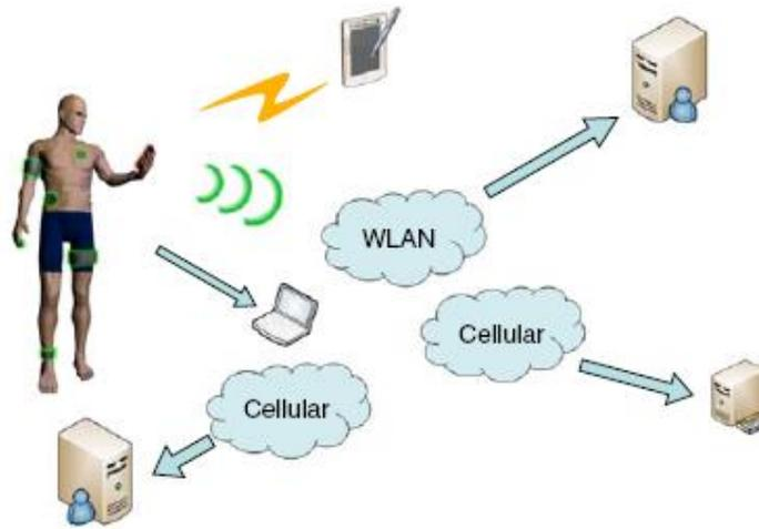
**Figure 5. Inter-WBAN communication architecture**
