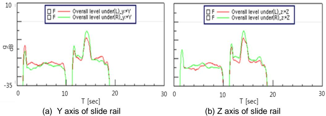
**Figure 13. Overall vibration level of the slide towards Y axis & X axis**
