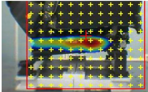
**Figure 8. Visualized noise during slide movement to rear position**
