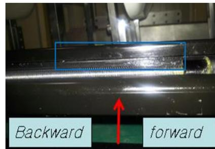
**Figure 2. Abraded portion in the rail occurred during slide movement**
