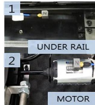
Figure 6. Position of sensor
