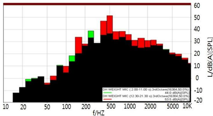
**Figure 10. 1/3 Comparison of noise level in CW and CCW in octave band**
