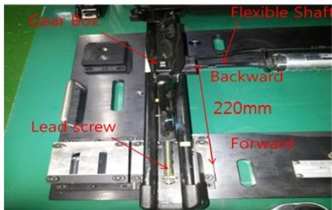
**Figure 1. Photos of seat sliding parts' structure**
