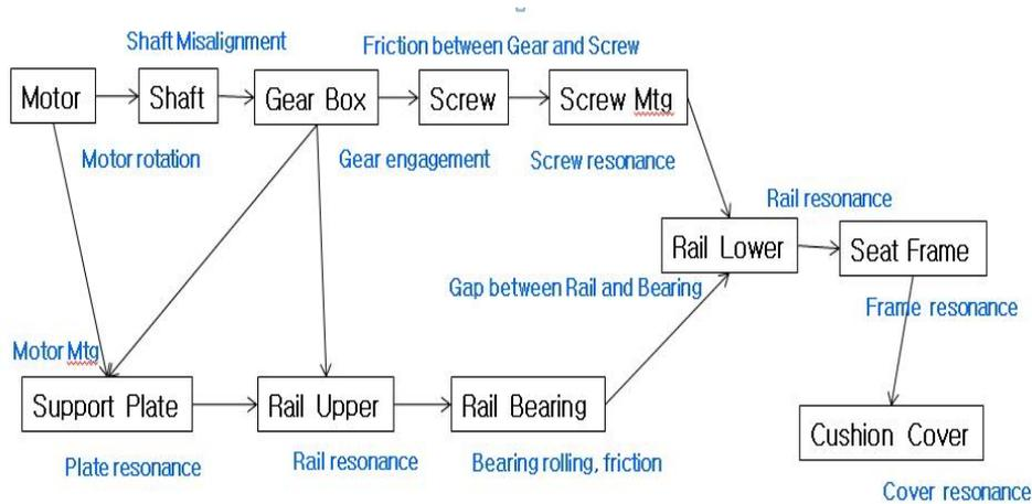
**Figure 7. Transmission route of noise and vibration**
