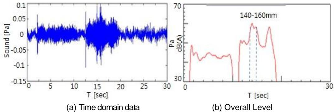
**Figure 9. Time domain data & overall level of the noise from the slide rail**
