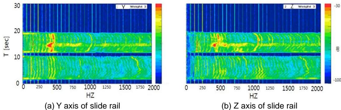
**Figure 14. Spectrum contour maps for Y axis and Z axis of slide rail**
