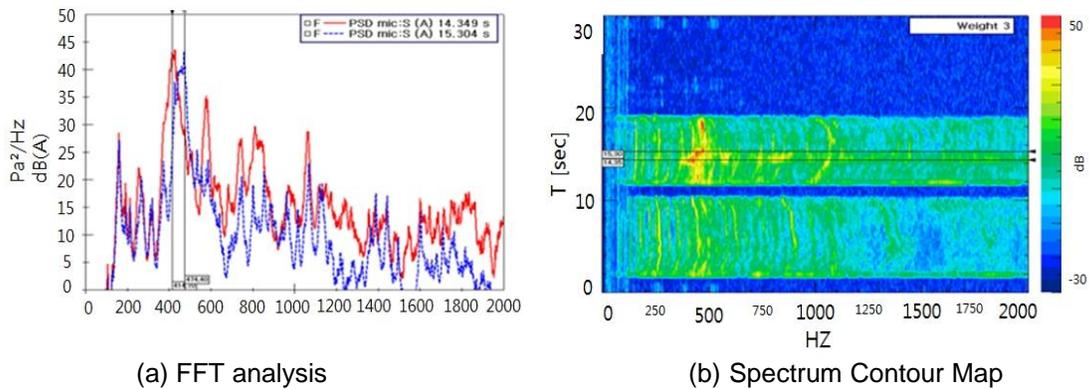
**Figure 11. FFT and Spectrum Contour Map of the seat**
