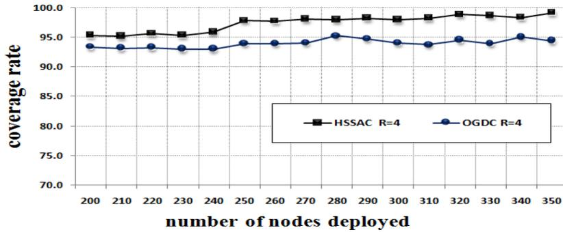
Figure 6. The Coverage Rate of the Active Sensor Set in Different Configurations (R=4)
