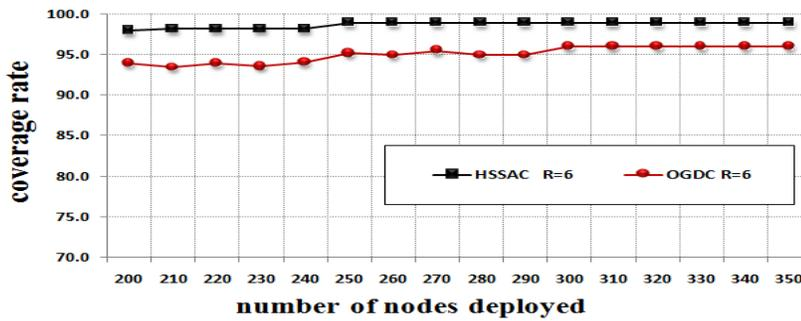
Figure 7. The Coverage Rate of the Active Sensor Set in Different Configurations (R=6)
