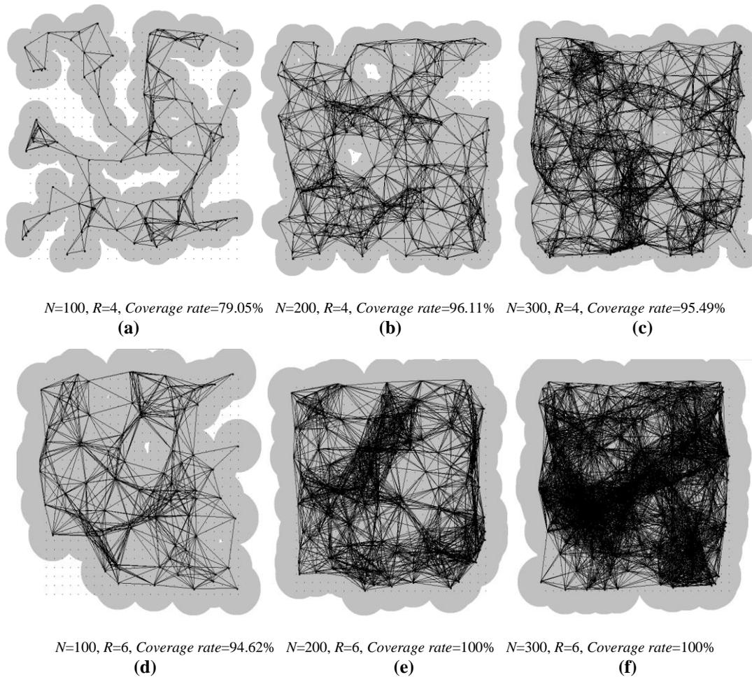
**Figure 5. The Coverage Rate for the Sensor Network (all Sensor Nodes are in Active Mode)**
