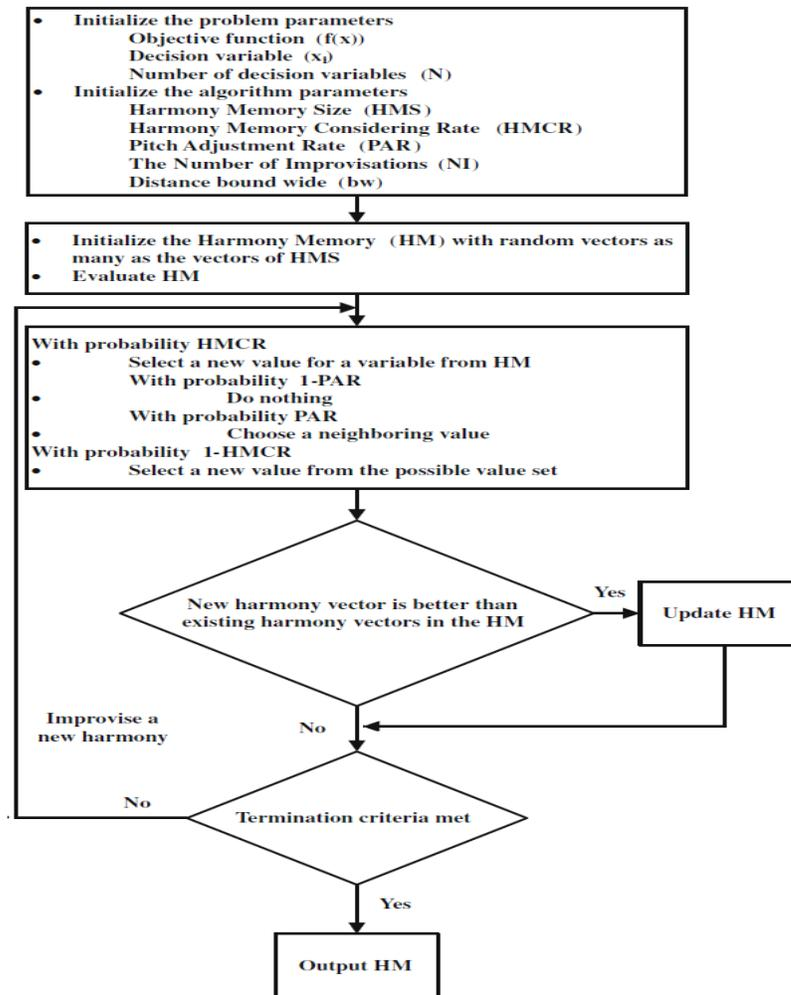
Figure 1. Block Diagram of HS Algorithm
