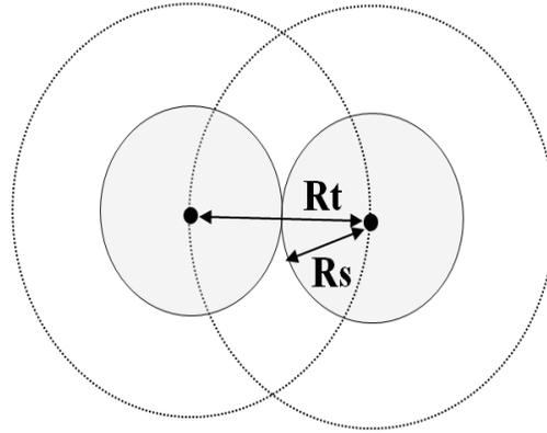
**Figure 2. The Transmission Radius of Sensor Nodes is assumed to be at Least Twice the Sensing Radius. then Coverage can Imply Connectivity**
