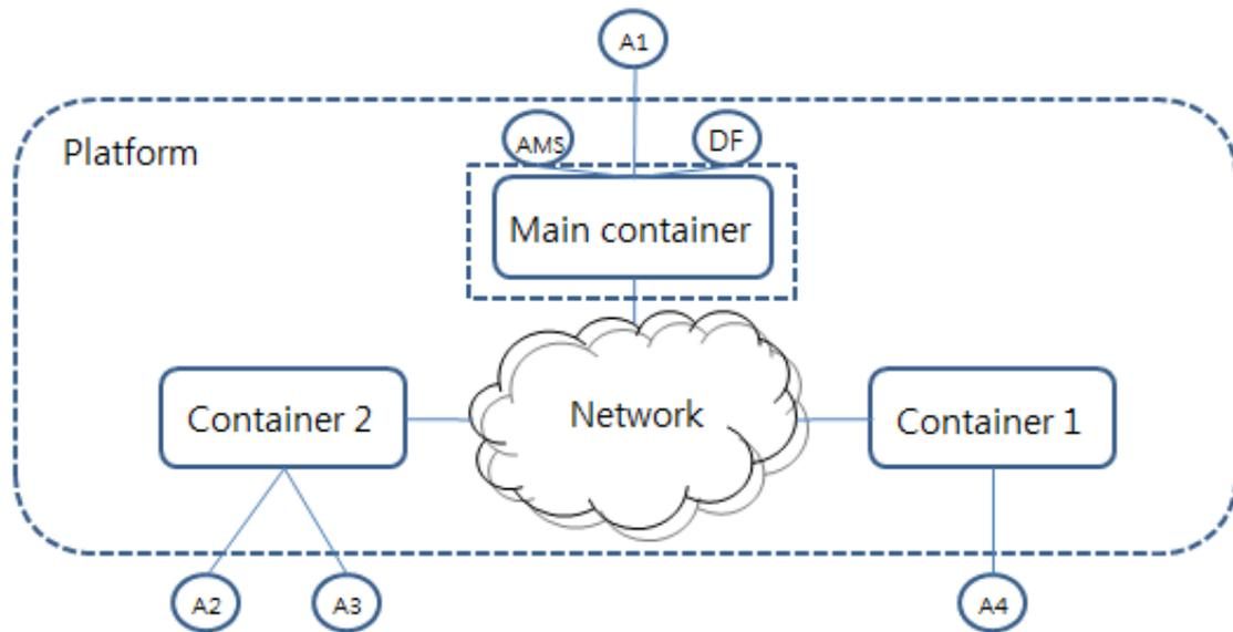
Figure 3. The Structure of JADE Framework
