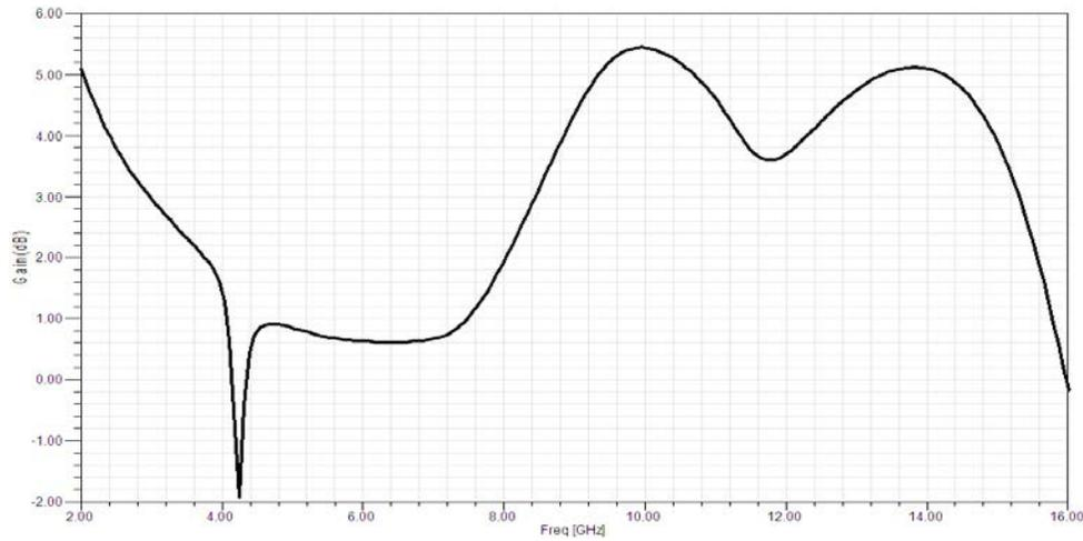
Figure 2. Measured Gain of the Designed Antenna
