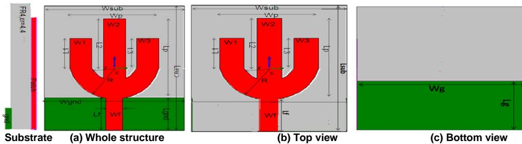
**Figure 1.1. Geometry of Designed TMP UWB Antenna (TMP)**
