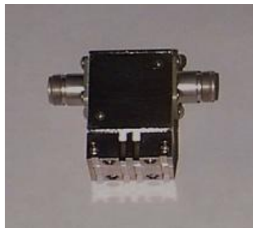
Figure 6. The Photo of the Isolator
