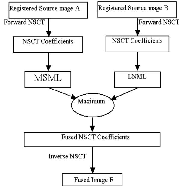
**Figure 3. Schematic Diagram of NSCT-based Fusion Algorithm**
