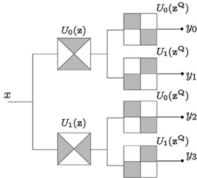
**Figure 2. NSDFB Constructed with Two-channel Fan Filter Bank**
