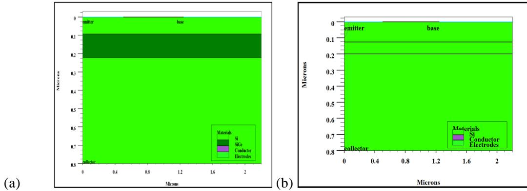
**Figure 2. (a) Strained Si<sub>0.88</sub>Ge<sub>0.12</sub> HBT (b) Simulated Si BJT for 100nm base Width**
