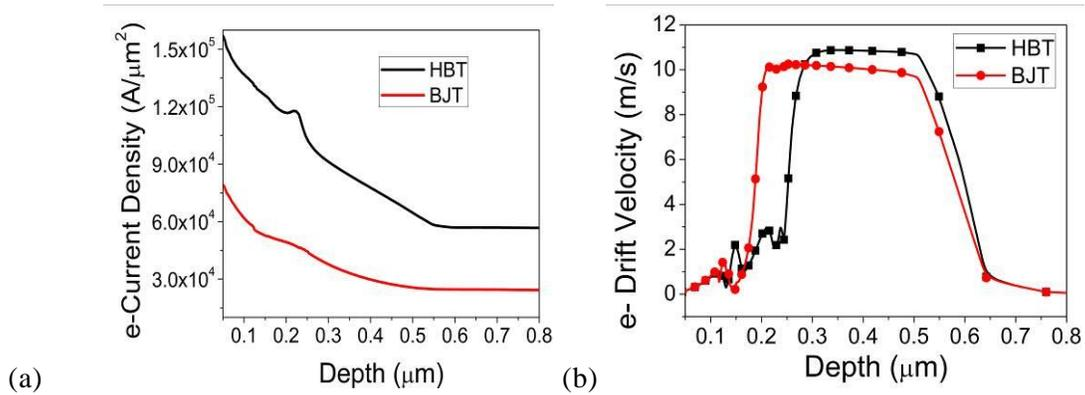
**Figure 4. (a) Vertical Electron Density Profiles of Si BJT & SiGe HBT at  $V_{BE}=0.7 \text{ V}$  and  $V_{CE}=2.0\text{V}$ , (b) Electron Velocity Profiles in the Base (100nm) of the SiGe-HBT Obtained by the DD Simulation at  $V_{BE}=0.7\text{V}$  and  $V_{CE}=2.0\text{V}$**
