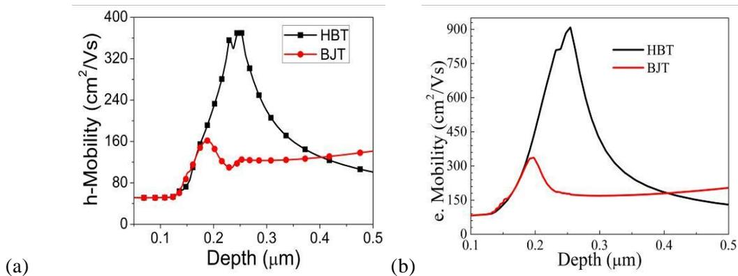
**Figure 5. (a) Vertical Hole Mobility of Si BJT & SiGe HBT at  $V_{BE}=0.7 \text{ V}$  and  $V_{CE}=2.0\text{V}$ , (b) Vertical Electron Mobility of Si BJT & SiGe HBT at  $V_{BE}=0.7 \text{ V}$  and  $V_{CE}=2.0\text{V}$**
