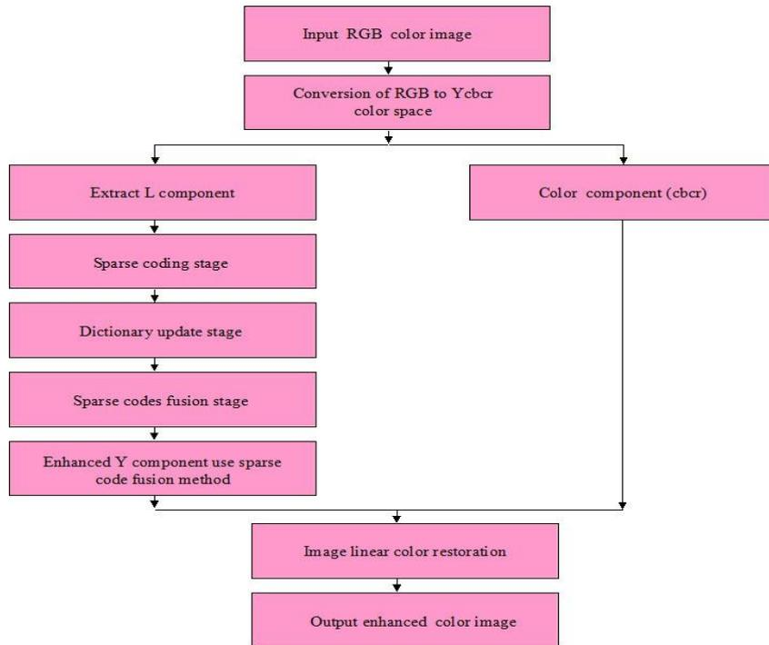
**Figure 1. A Block Diagram of the Proposed Sparse Code Fusion Method**
