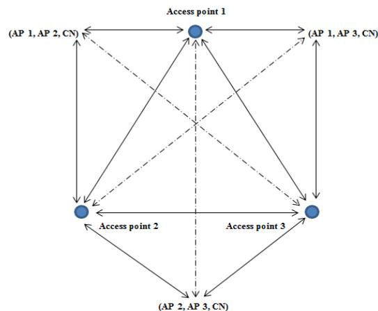
Figure 5. Three Wi-Fi and Cellular Network Combination Fingerprint
