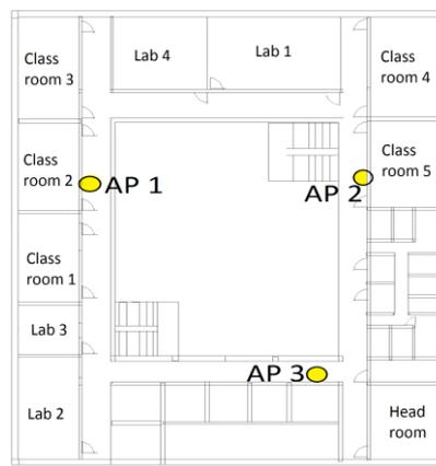
Figure 4. Building with Three APs Position
