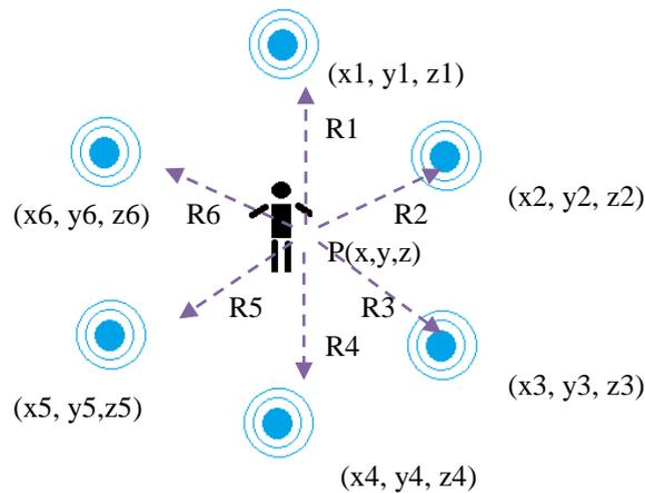
**Figure 11. Smart Device Position  $P(x, y, z)$  Signal Compare with Predefined Points**
