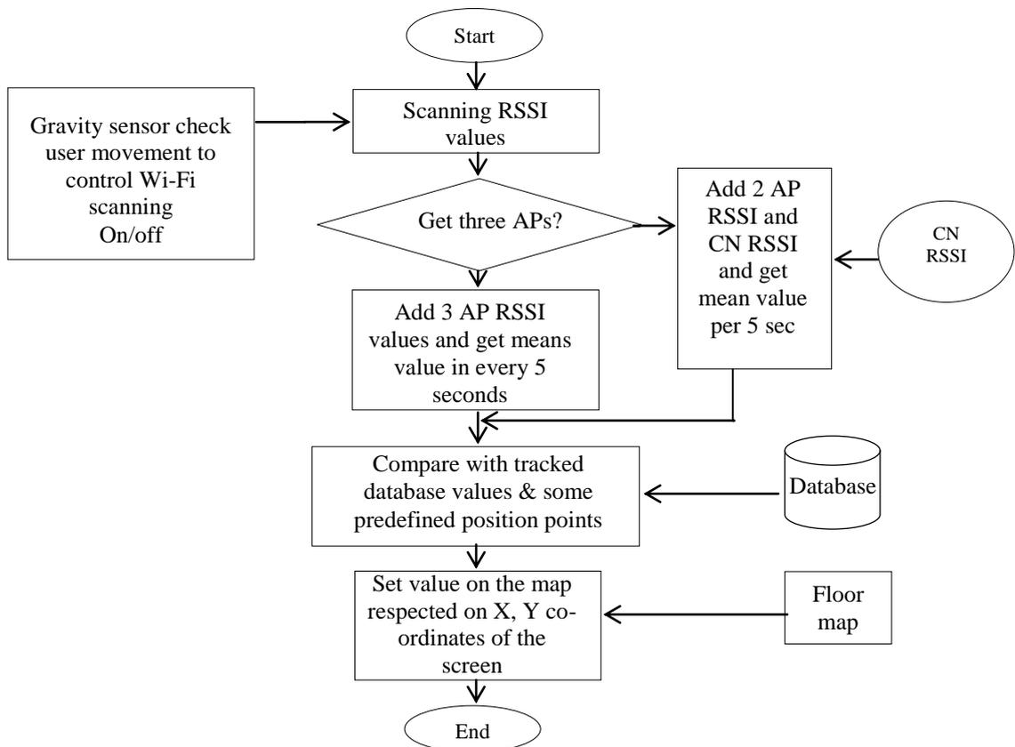
**Figure 3. Flowchart of Indoor Positioning Algorithm**
