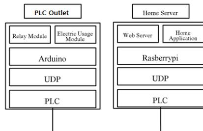
Fig. 2. Structure of Smart Outlet Communication
