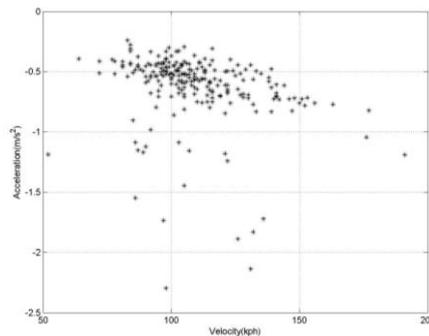
Fig. 1. Deceleration distribution in practical braking
