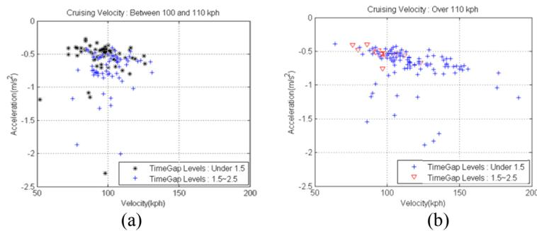
**Fig. 3** Distributions of deceleration vs. vehicle speed: (a) cruising velocity between 100kph and 110kph, (b) cruising velocity over 110kph
