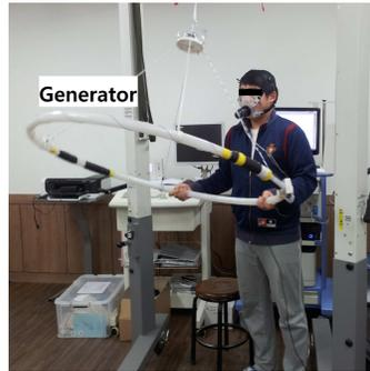
**Fig. 3.** The experimental setup for metabolic assessment of exercise load required to steer the hula-hoop generator.
