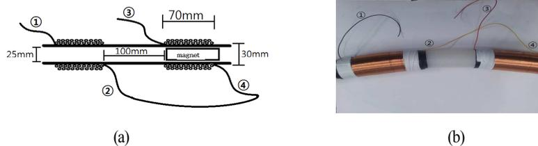
**Fig. 1.** (a) schematic diagram, (b) The electromagnetic configuration of the hula-hoop generator.
