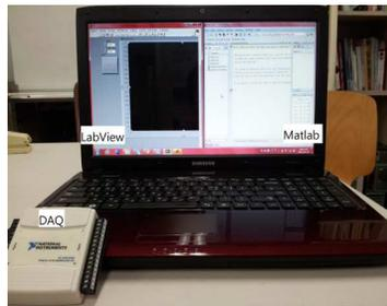
**Fig. 2.** The data acquisition device and software to measure the generator output.
