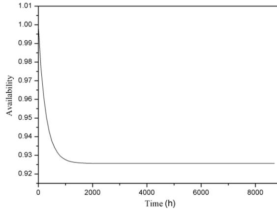
**Fig. 2.** Transient availability of subsea annular blowout preventer
