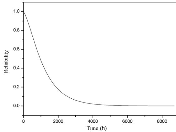
**Fig. 3.** Transient reliability of subsea annular blowout preventer
