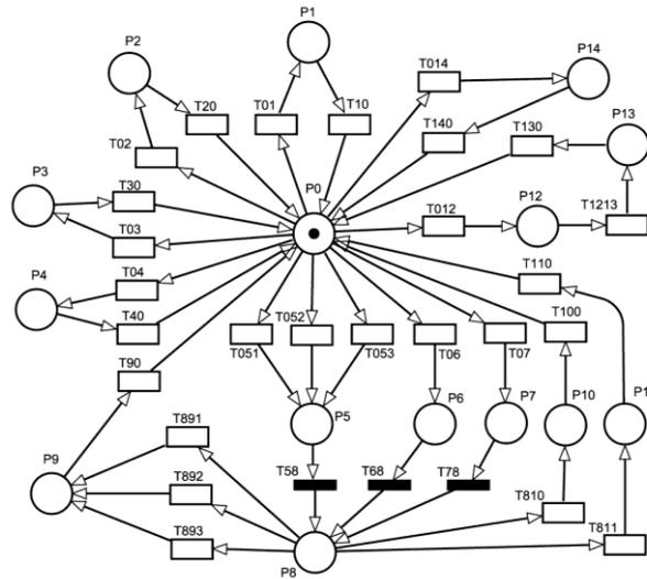
Fig.1. Stochastic Petri nets model of subsea annular blowout preventer
