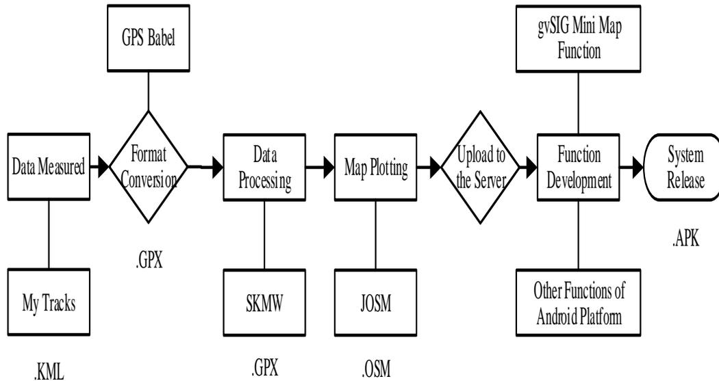
**Figure 2. Main Work Flow Chart of JiuFeng Guiding System**
