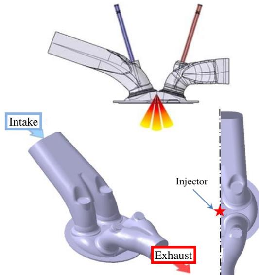
**Figure 6. Computational Geometry of Cylinder Head and Ports**
