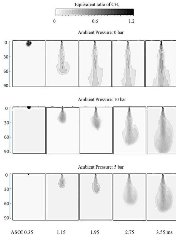
**Figure 8. Transient Modeling on CH<sub>4</sub> Jet Penetration and Mixture Formation in a Constant Volume Chamber ( $P_{inj}$ : 85bar,  $T_{ambient}$ : 20°C)**
