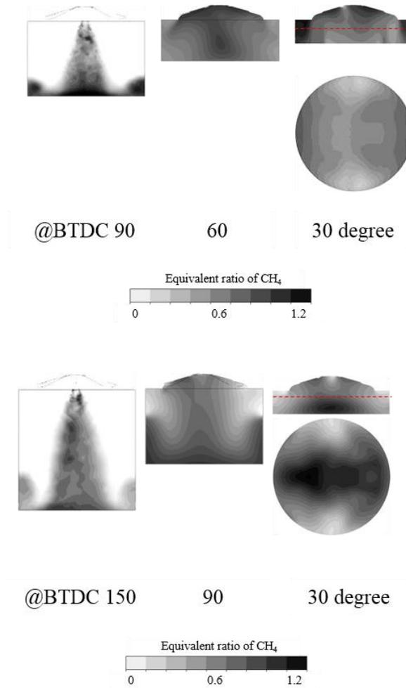
**Figure 11. CH<sub>4</sub> Mixture Formation in Engine Cylinder (CH<sub>4</sub>: 10mg & CH<sub>4</sub>: 23mg)**
