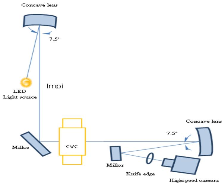
**Figure 1. Schematic Diagram of Schlieren Optical System**
