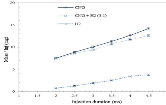
**Figure 7. Mean Mass Flow Rate versus Injection Duration**
