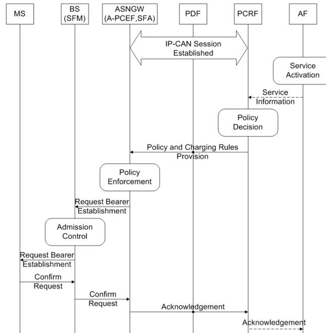
Figure 2. Dynamic QoS Setup based on PCC
