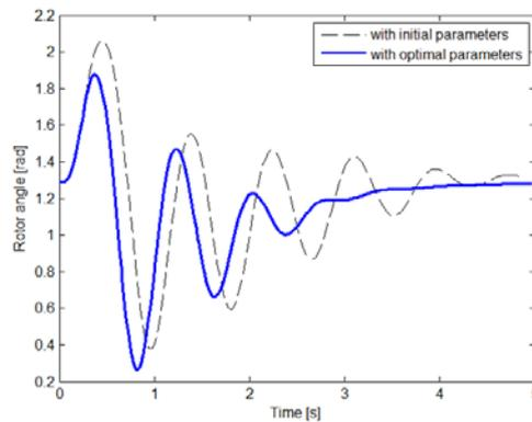
**Fig. 2.** Generator rotor angle [rad]
