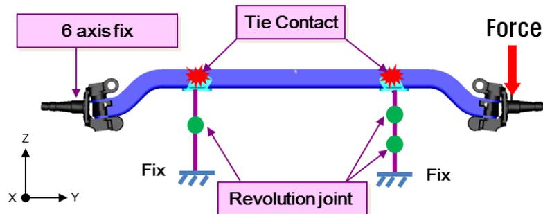
Fig. 2. Strength analysis boundary condition modeling
