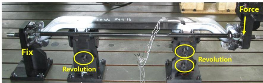
Fig. 1. Strength test evaluation environment
