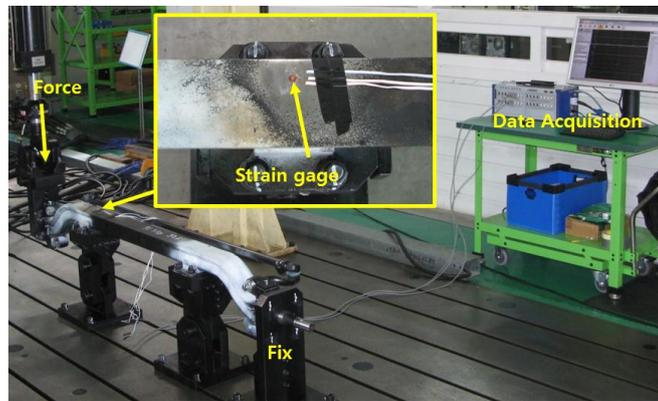
**Fig. 3.** Strain verification test settings
