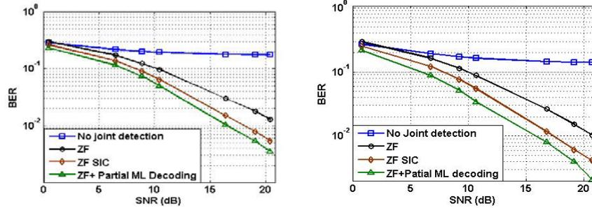
Fig. 1. BER performance comparison of joint detection algorithms when Three and four BSs are cooperated.
