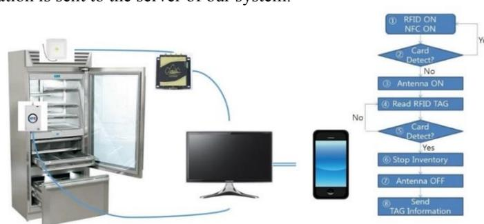
Fig. 1. Smart refrigerator operation algorithm
