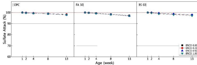
Fig. 3. Resistance to sulfate attack with age depending on ERCO dosages
