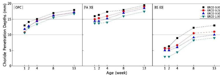
**Fig. 2.** Resistance to chloride penetration with age depending on ERCO dosages
