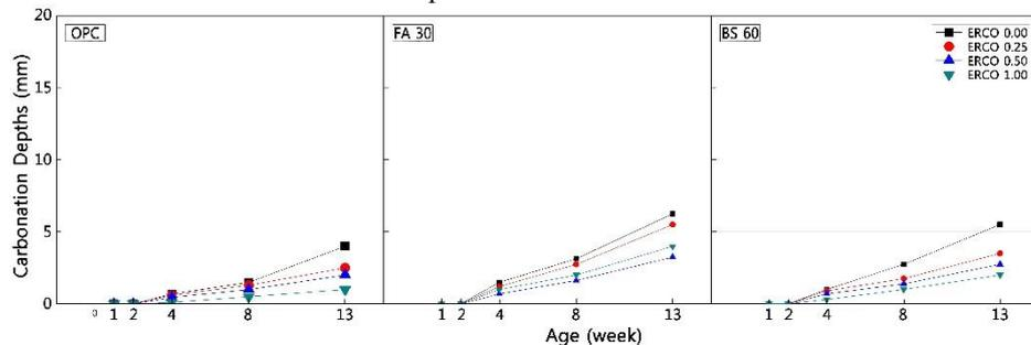
**Fig. 1.** Carbonation depth of the concretes with age depending on different admixtures and ERCO dosages
