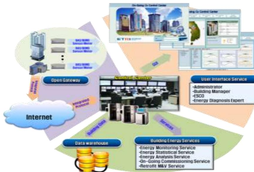
**Fig. 1.** A configuration of Building Group Management Service Framework for On-Going Commissioning
