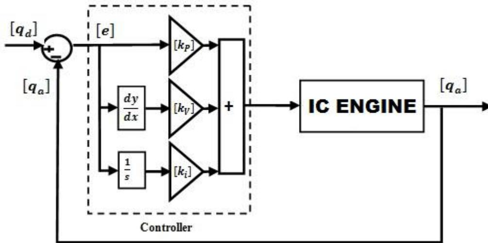
Figure 11. Block Diagram of PID Control of IC Engine
