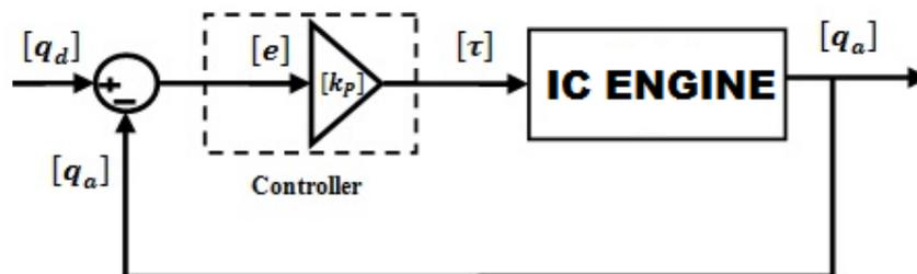
**Figure 4. Block Diagram of Proportional Controller**
