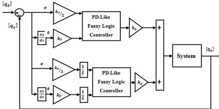
Figure 21. Design PID like Fuzzy Controller
