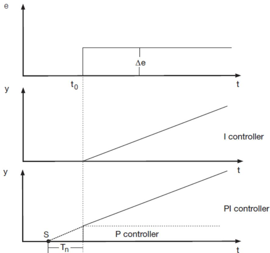
**Figure 10. Step Response of a Proportional-Integral (PI) Controller**
