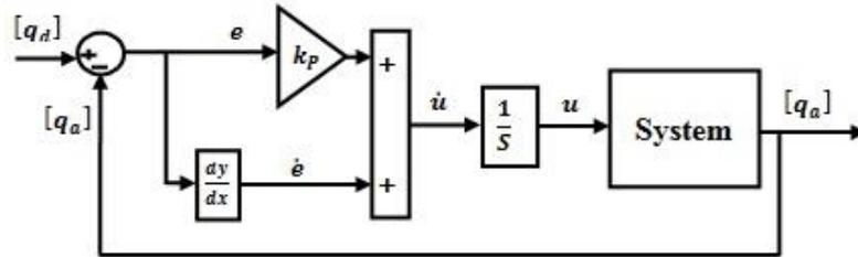
Figure 19. Design PI Controller Based on PD Controller
