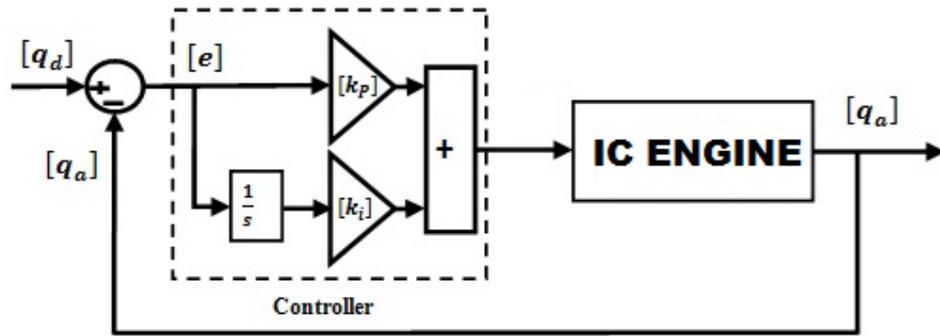
**Figure 9. Block Diagram of PI Control of IC Engine**
