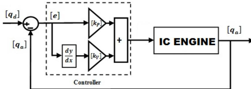
**Figure 5. Block Diagram of PD Control of IC Engine**
