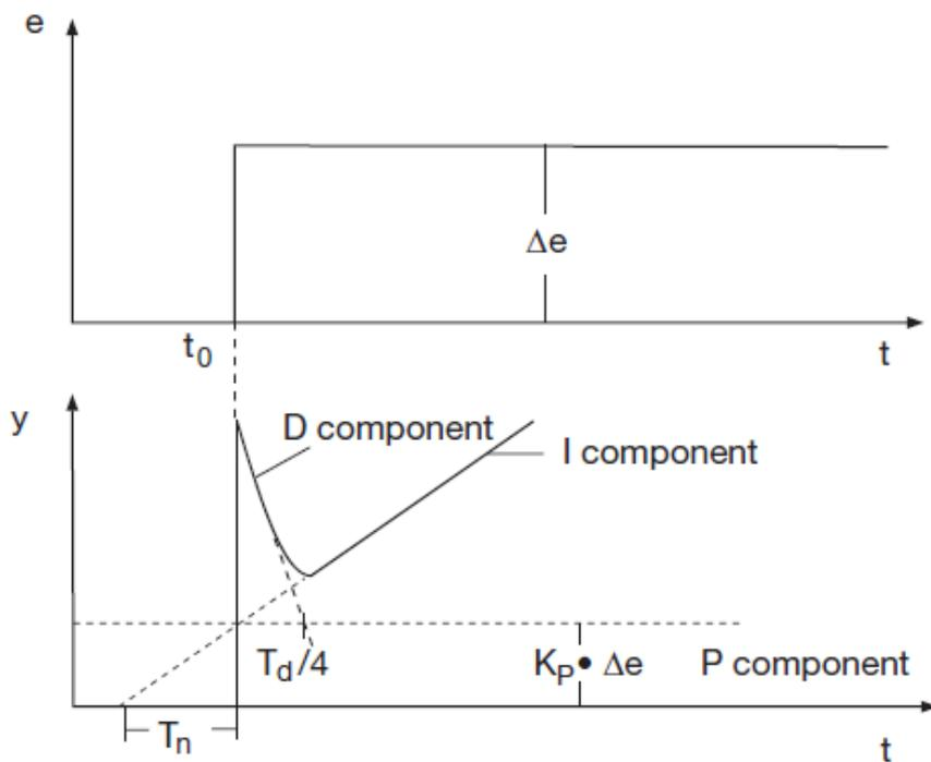
Figure 12. Step Response of a Proportional-Integral-Derivative (PID) Controller
