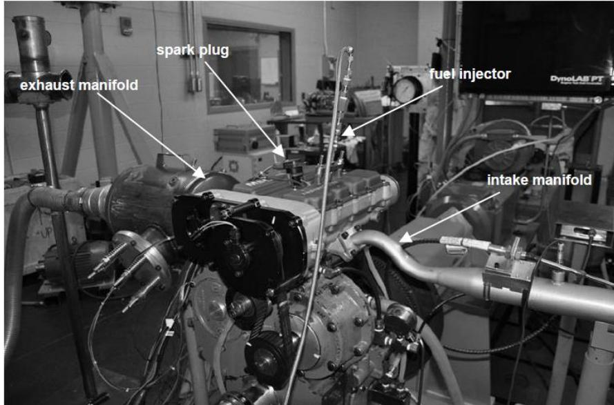
**Figure 3. Test Engine**
