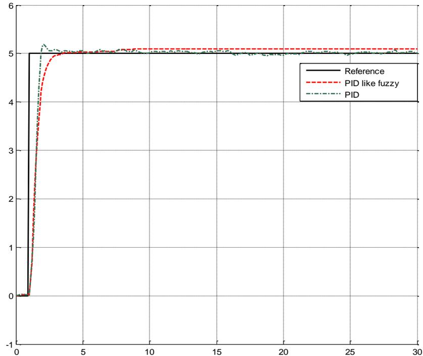
**Figure 23. Tracking Data: PID like Fuzzy Controller and PID Controller in Presence of Uncertainty**
