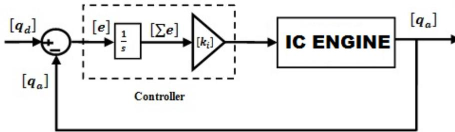
**Figure 7. Block Diagram of Integral Control of IC Engine**
