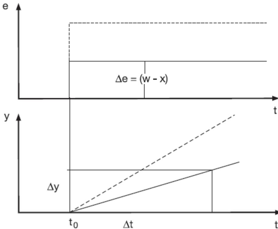
**Figure 8. Step Response of an Integral (I) Controller**
