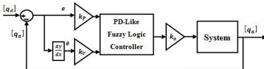
**Figure 18. PD-like Fuzzy Logic Controller**
