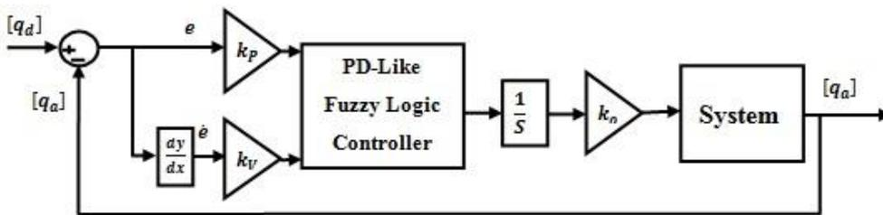
Figure 20. Design PI like Fuzzy Controller Based on PD like Fuzzy Controller
