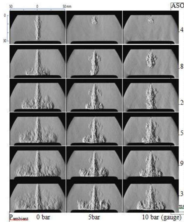
**Figure 6. Schlierenimages of the transient CNG impingement jet under different ambient pressure( $P_{inj}$ : 85bar,  $T_{ambient}$ : 20°C)**
