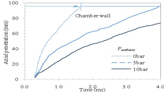
**Figure 2. CNG free-jet penetration**
