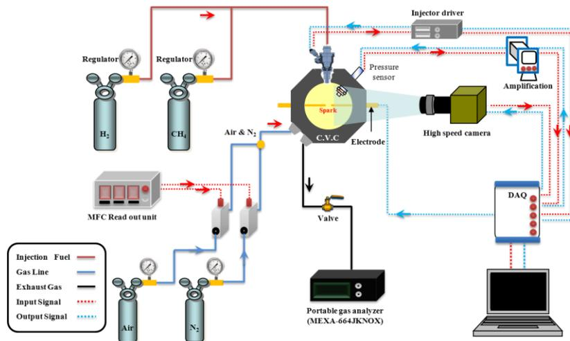
**Figure 1. Schematic diagram of experimental apparatus with a constant volume chamber**
