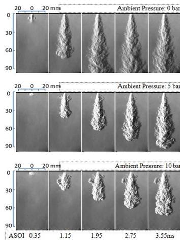
**Figure 3. Schlieren images of the transient CNG free jet under different ambient pressure**
