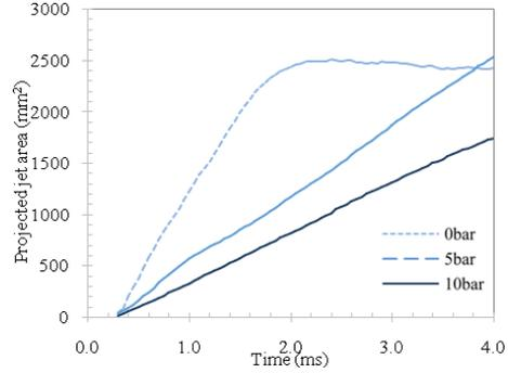
Figure 5. CNG free-jet projected area
