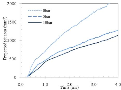
**Figure 8. CNG Projected area**
