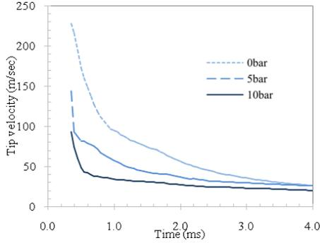
Figure 4. CNG free-jet tip velocity
