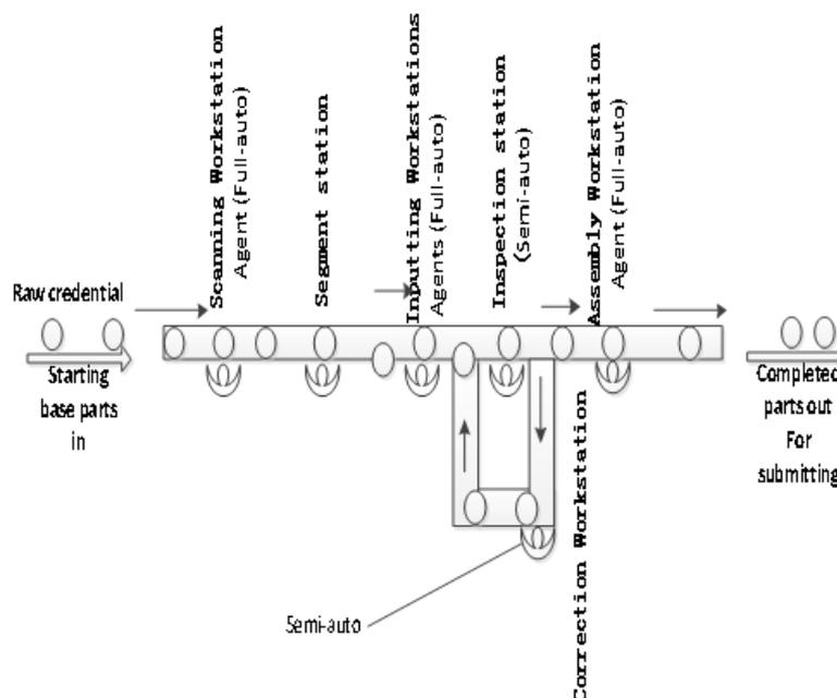
**Figure 12. Model of Data-BPO Production Line**
