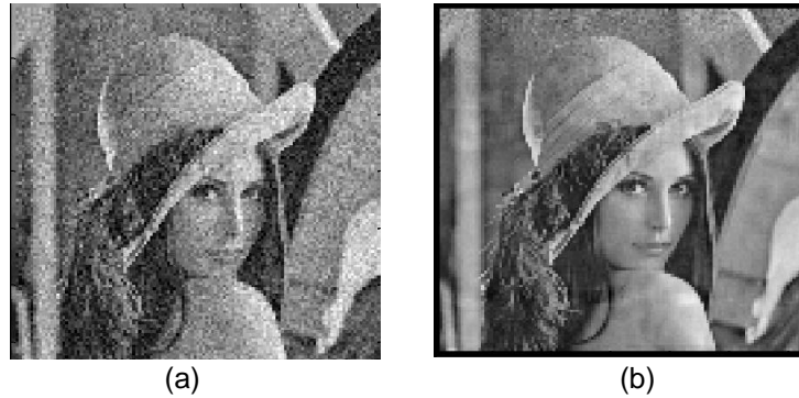
Figure 3. Restoring when the Reference Random Noise is a Shifted and Scaled Version of the Disturbance Added to the Image: (a) the Input Image with Additive Noise (b) the Restored Image
