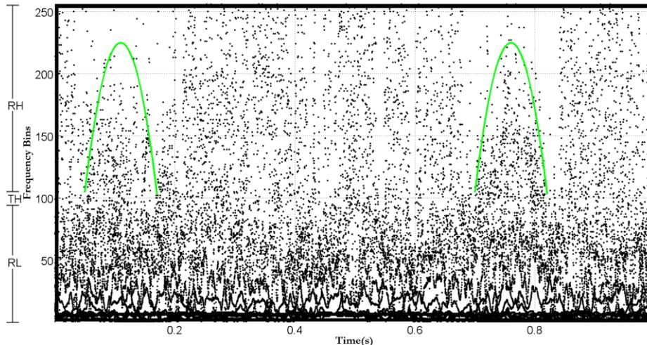
**Figure 4. Hilbert Spectrum of the Doppler Ultrasound Signal**
