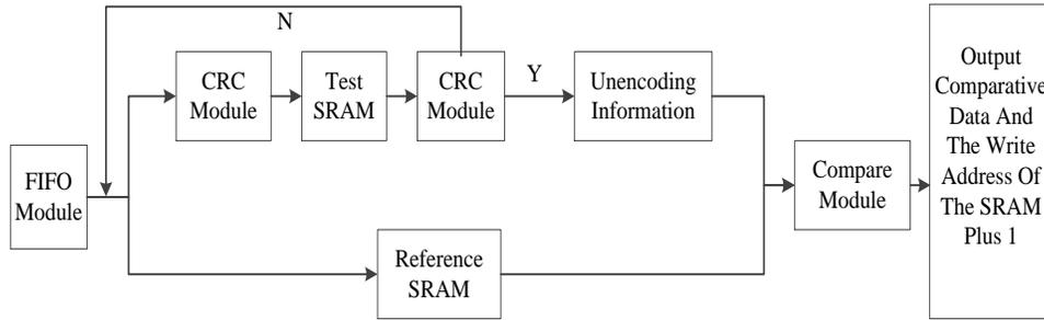
**Figure 3. CRC Checking Reinforcement Flow Chart**
