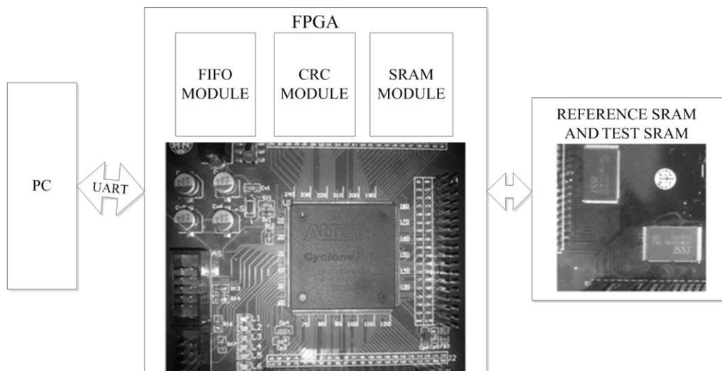
Figure 1. The Overall Structure of the Test System
