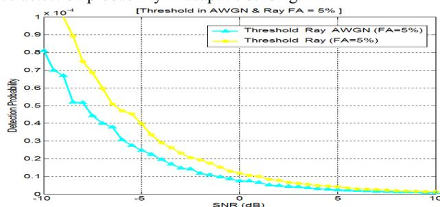
Fig. 2. Compare Detection Threshold Probability between AWGN and Ray in FA=5%
