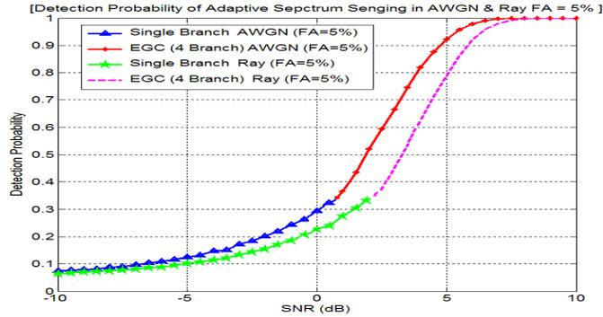
Fig. 4. Compare Detection Probability of Adaptive Spectrum Sensing between AWGN and Ray.
