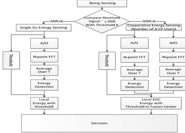
Fig. 1. Proposed Adaptive Sensing Model.
