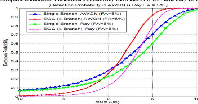
Fig. 3. Compare Detection Probability Single Sensing with 4 branch of Cooperative Sensing and AWGN with Ray in Threshold FA=5%.
