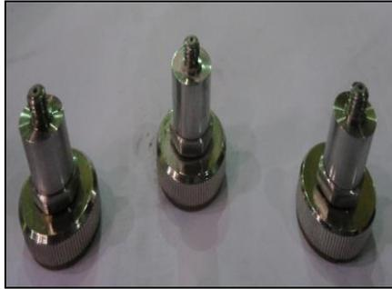
**Figure 5. The ICP Type Acceleration Sensors**
