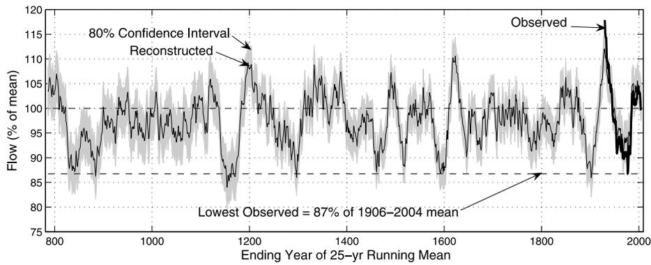
**Figure 2.** Time series plot of 25-year running mean of reconstructed flows. Flows are plotted as percentage of the 1906–2004 mean of observed natural flows (18.53 billion cubic meters, or 15.03 million acre-ft). Confidence interval derived from 0.10 and 0.90 probability points of ensemble of 1000 noise-added reconstructions. Horizontal dashed line is lowest 25-year running mean of observed flows (1953–1977).
