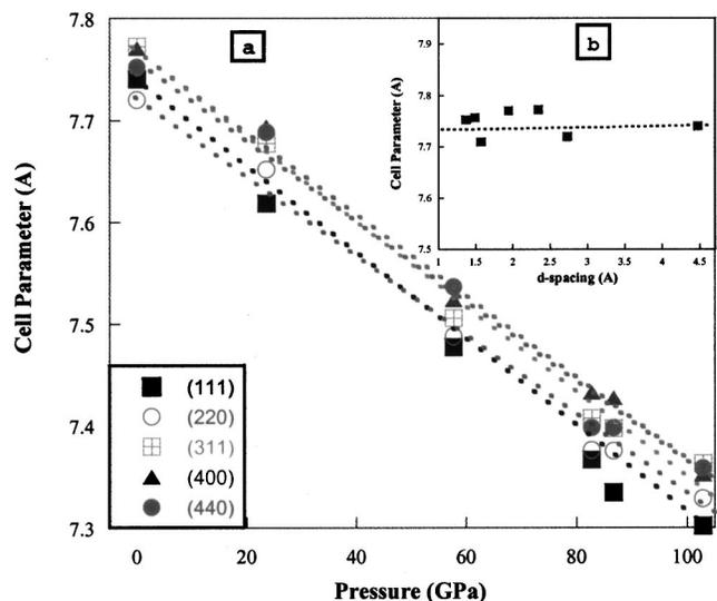
FIG. 3. (a) Pressure dependence of the cell parameter ( $a$ ) calculated from the observed diffraction planes of nanocrystalline spinel  $\text{Si}_3\text{N}_4$  upon release of pressure. Note: We did not use some broad low intensity peaks, as described in Fig. 1(b). (b) Correlation between  $d$  spacing and cell parameter ( $a$ ) of the pressure-quenched nanocrystalline spinel  $\text{Si}_3\text{N}_4$ .
