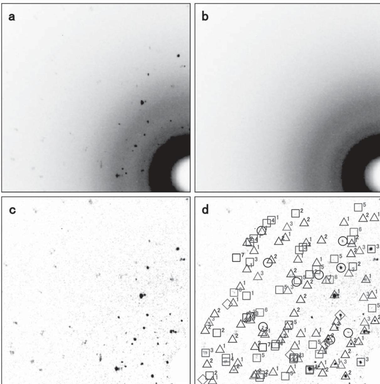
**FIGURE 3.** Four XRD pattern frames. (a) A CCD XRD pattern frame of the rock thin section on the slide glass. (b) A CCD XRD pattern frame of the slide glass without thin section. (c) The XRD pattern of the rock thin section from which the background of the slide glass is subtracted. (d) The XRD pattern in which the spot origins are assigned to each mineral. Open circle specifies a coesite; open diamond = a quartz; open triangles = three garnets; open squares = eight omphacites.
