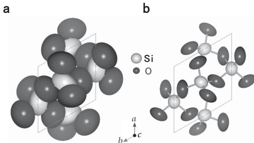
**FIGURE 9.** Crystal structures of quartz illustrated in the form of thermal ellipsoids at 99.99% probability. (a) Quartz determined by this study for Sulu UHP rocks. (b) Natural quartz reported by Kihara (1990) at room conditions.
