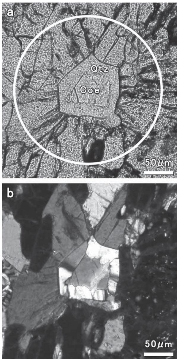
**FIGURE 1.** Coesite mantled by retrograde quartz crystals in the Sulu UHP rock. (a) Photomicrograph under plane-polarized light. A circle of 250  $\mu\text{m}$  diameter shows the area irradiated by X-rays. (b) Photomicrograph under cross-polarized light.
