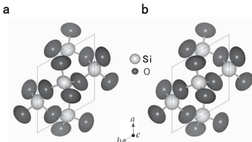
**FIGURE 10.** Crystal structures of quartz in the Oomine granite illustrated in the form of displacement ellipsoids at 99.99% probability. (a) Quartz determined by the conventional method using an extracted single crystal on a goniometer head. (b) Quartz determined by the new method using a rock thin section.
