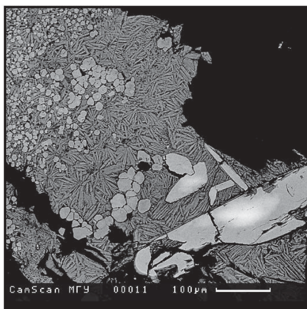
FIGURE 1. BSE image of euhedral clinopyroxene crystals, coexisting with garnet (small euhedral grains in the matrix), produced in the run 939 ( T = 1480 °C, P = 7 GPa). CamScan electronic microscope.
